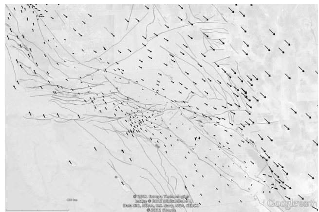
Figure 6. GPS vectors plotted for southern California relative to station CHIL in the San Gabriel Mountains. Fault traces are from UCERF-2 [4].
