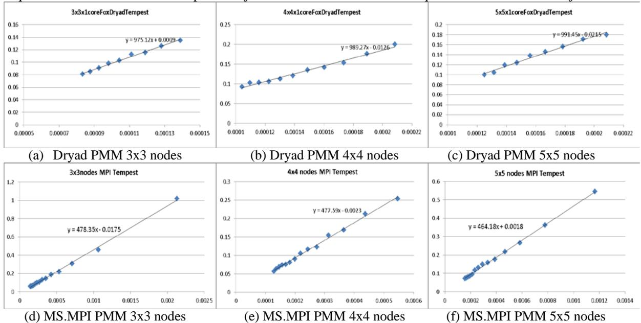
Figure 4: (a)(b)(c) plots parallel overhead vs.  $(\sqrt{N} * (\sqrt{N} + 1)) / (4 * M)$  of Dryad PMM using different number of nodes on Tempest. (d)(e)(f) plot parallel overhead vs.  $(\sqrt{N} * (1 + \log_2^{\sqrt{N}})) / (4 * M)$  of MS.MPI PMM on Tempest.
