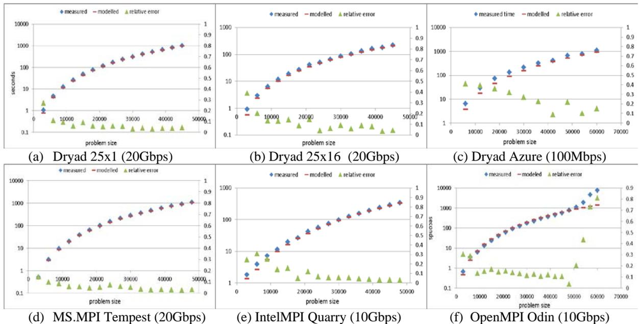
Figure 6: comparisons of measured and modelled job running time using different runtime environments. (a) Dryad PMM on 25 nodes on Tempest with 20Gbps network. (b) Dryad PMM with 25nodes with 16 cores per node on Tempest with 20Gbps network. (c) Dryad PMM on 100 small instances on Azure with 100Mbps network. (d) MS.MPI PMM on 25 nodes on Tempest with 20Gbps network. (e) IntelMPI PMM on 100 nodes on Quarry with 10Gbps network. (f) OpenMPI PMM on 100 nodes with 10Gbps network.
