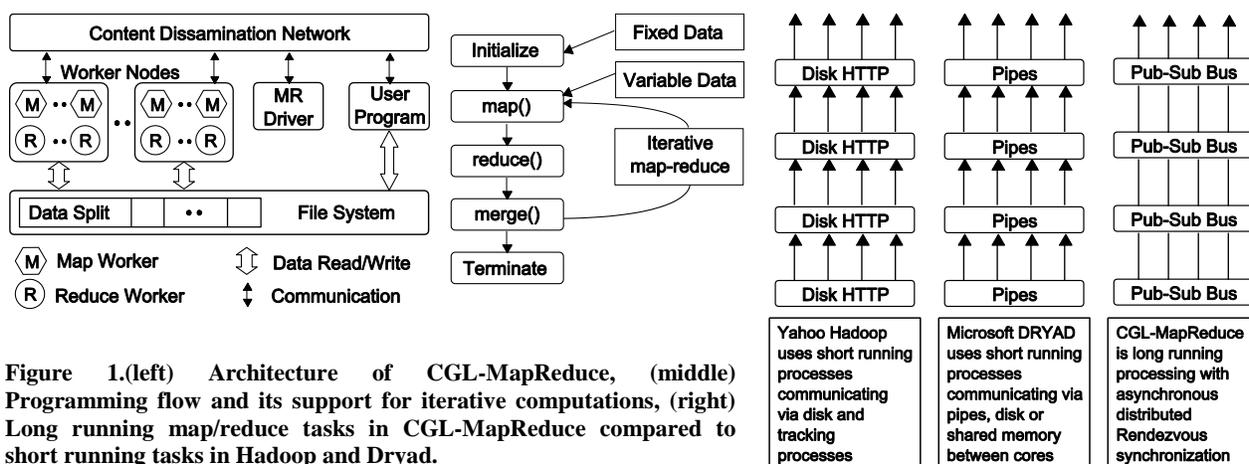
Figure 1.(left) Architecture of CGL-MapReduce, (middle) Programming flow and its support for iterative computations, (right) Long running map/reduce tasks in CGL-MapReduce compared to short running tasks in Hadoop and Dryad.
