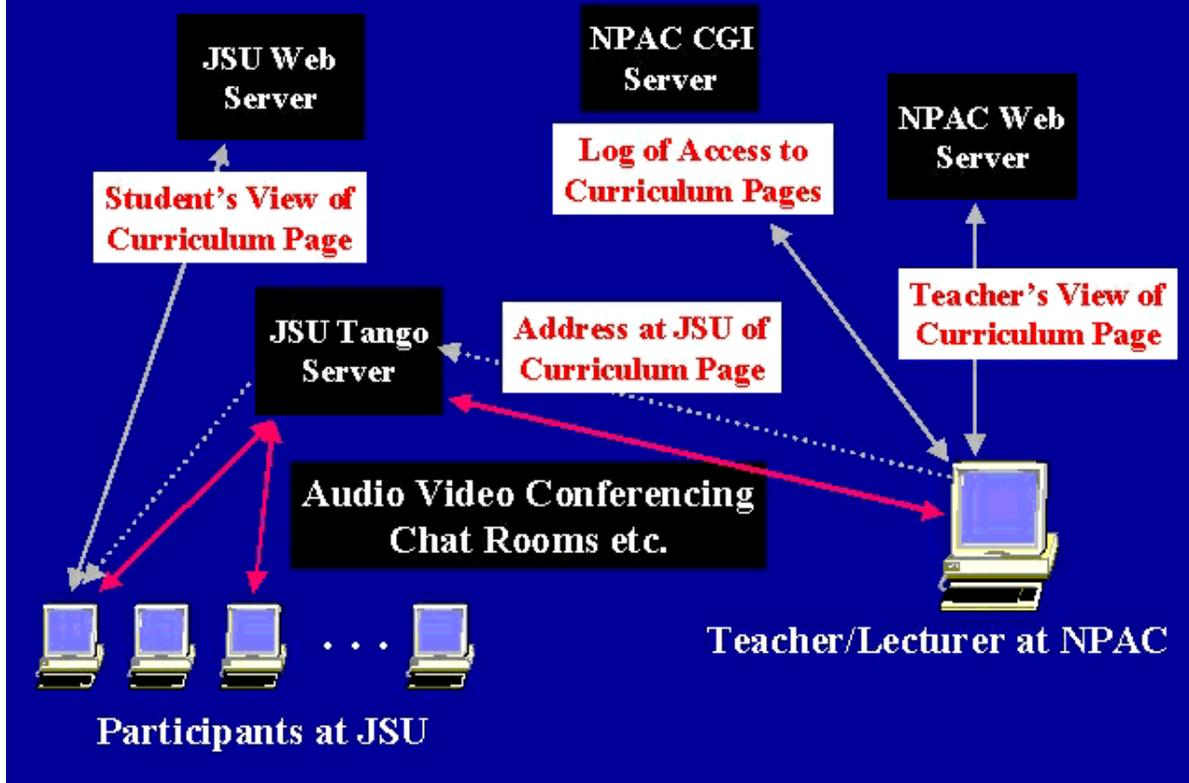
**Figure 9: Dual-server Network Architecture**
