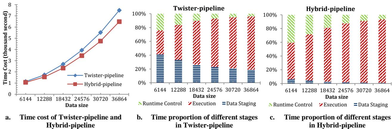
**Figure 6 Performance comparison chart between Twister-pipeline which only use Twister as MapReduce runtime and Hybrid-pipeline use both Hadoop and Twister. Input data size is increased from 6144 to 36864 and core number is fixed to 768**
