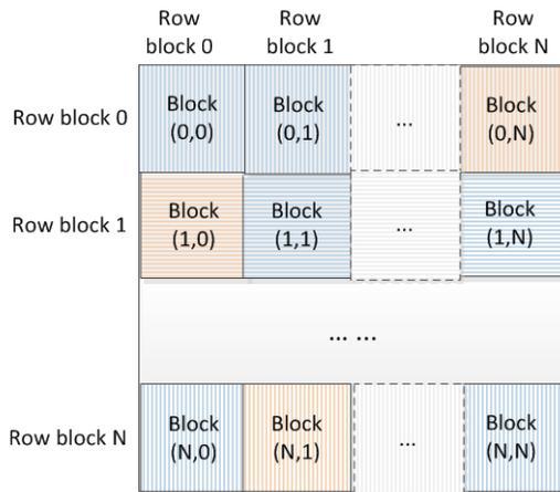
**Figure 5 Architecture of parallel pairwise sequence alignment**
